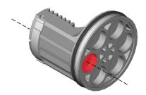
The drive pistons are not symmetrical due to the attached racks. In order to ensure optimal flow of force and minimize internal wear, the springs must be installed according to the following installation schemes.
